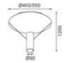
Item No Product size Power 51752C Ø400*1200mm 24W 51753C Ø550*1200mm 36W Anodized Brown+ Sand White
